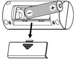
Remove the cover to insert the battery
