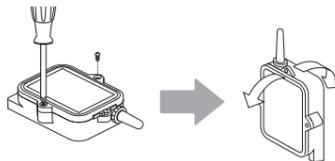
2. Insert the battery in its tube and place in unit as in diagram.
