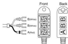
3. Connect the Sensor Adaptor to the RTR-52Pt Logger's Sensor Jack.
